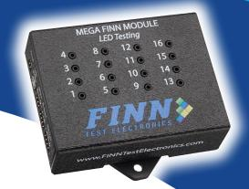
The module(s) may be implemented into functional, in-circuit or stand alone systems, using either a USB or serial interface.
